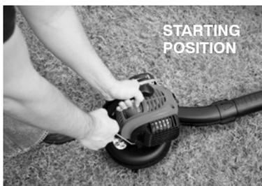
**WARNING:** When starting engine, hold the unit as illustrated. Do not set unit on any surface except a clean, hard area when starting engine or while engine is running. Debris such as gravel, sand, dust, grass, etc. could be picked up by the air intake and thrown out through the discharge opening, damaging the unit or property, or causing serious injury to bystanders or the operator.
