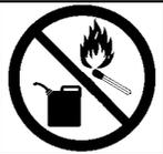
**WARNING:** Fire hazard. Never mix, pour, or store gasoline or use the unit near a flame or sparks (including smoking, open flames, or work that can cause sparks).
