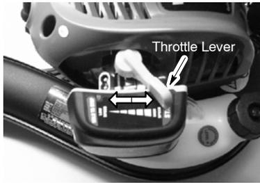
7. To stop engine, move the throttle lever to the STOP
