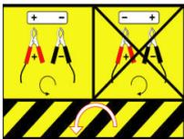
Polarity reversal of the bandsaw blade grinder when connected to a 12-volt battery.
